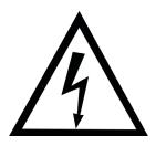
This internal component uses an AC current higher than 42.4V peak A.C. Do not touch this component if the ME Equipment is energized.
